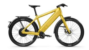
Both resulting in a new frame, hence the ST7. By the way, the battery cover on the left side is now made of aluminium and beautifully integrated in the downtube, which is an evolutionary step from the rubberlined one that was combined with a plastic cover below, which bulged in time and was not waterproof.
